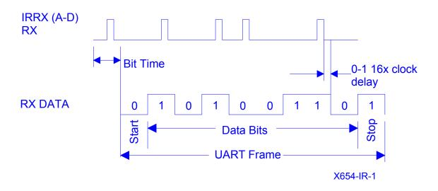
Infrared receive timing
