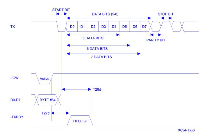
Transmit ready timing in FIFO mode
