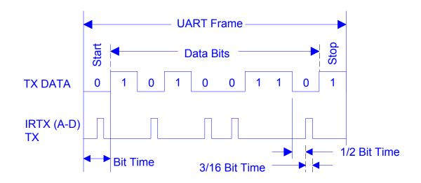
Infrared transmit timing
